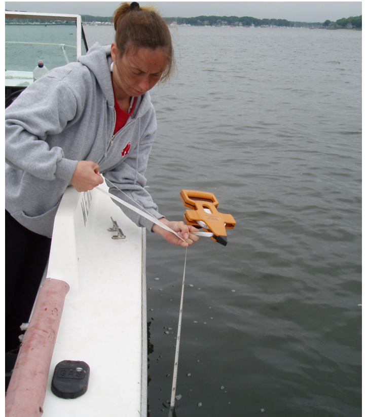
Jessica Morgan of NBEP uses a secchi disk to measure water clarity in Narragansett Bay. Photo: NBJ
