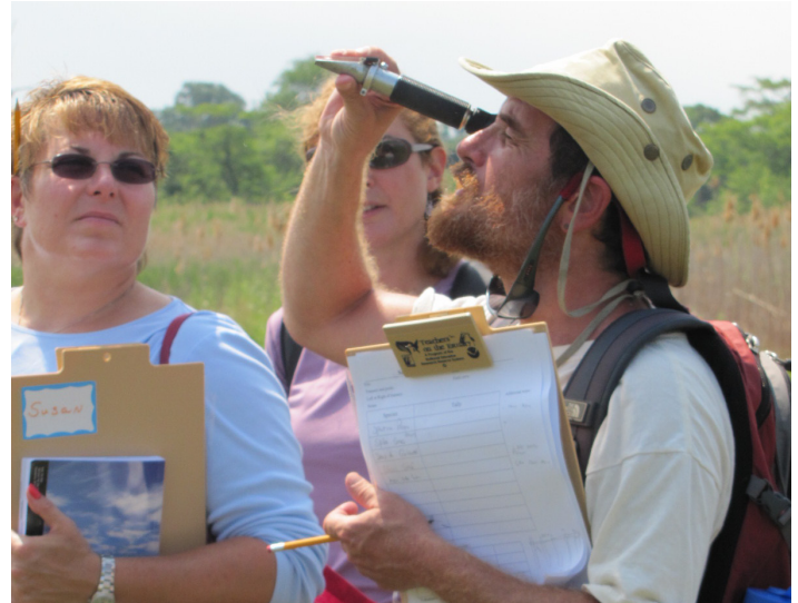
Teachers learn how to use a specrometer to measure salinity. Photo: Maureen Dewire, NBNERR.
